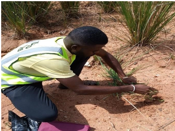
Figure 2.2: Vetiver rooted soil sample
